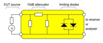
Fig. 1 Simplified limiter schematic
