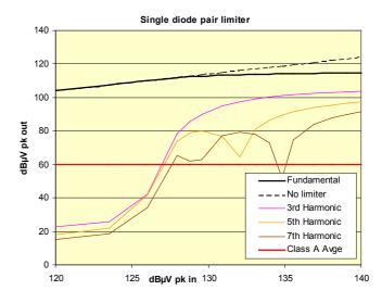
Figure 5 Harmonic output vs. input of the single pair limiter
