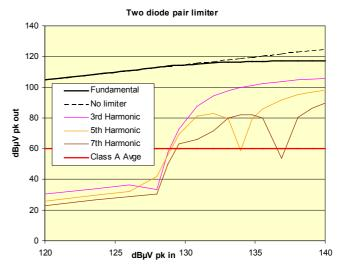
Figure 6 Harmonic output vs. input of the dual pair limiter
