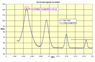
Fig. 4 The lower frequency fundamental and harmonics
