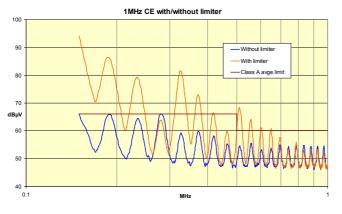
The limiter creates something like a 20dB increase in the low order harmonics, more than enough to make the product into a clear test failure. The amplitude of the low-frequency signals can be seen in Fig. 4 which shows the spectrum between 25kHz and 200kHz. For a standard CISPR 22 test, the signals below 150kHz would never be investigated.
