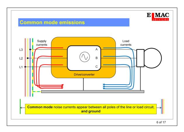
By contrast, common mode currents **do** flow in the earth structure. It is harder to see the coupling path and the source for these currents, until you realise that both the drive or converter and its load exhibit parasitic coupling components to the earth structure (next page).
