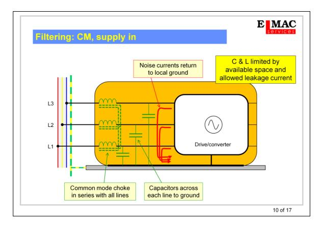
Conventional mains filters almost always will incorporate a common mode choke and capacitors from each line to the earth return, and supply filters for power drives and converters are no exception. In fact, if the module itself does not contain adequate filtering then a significant improvement in EMC performance can be obtained just by including capacitors to earth from each supply line, directly at the input terminals of the unit.
