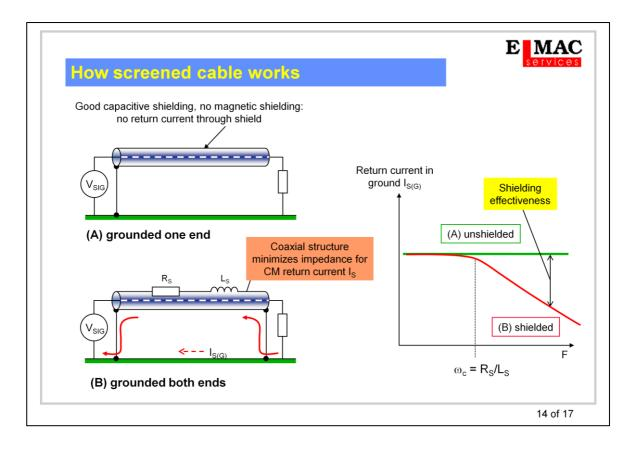
For low frequencies an overall screen, grounded only at **one** end, provides good shielding from capacitively coupled interference. In the case of high dV/dt on the inner wires this may be useful in some circumstances but it doesn't prevent earth currents, and the extra capacitive load on the output has to be accounted for.
