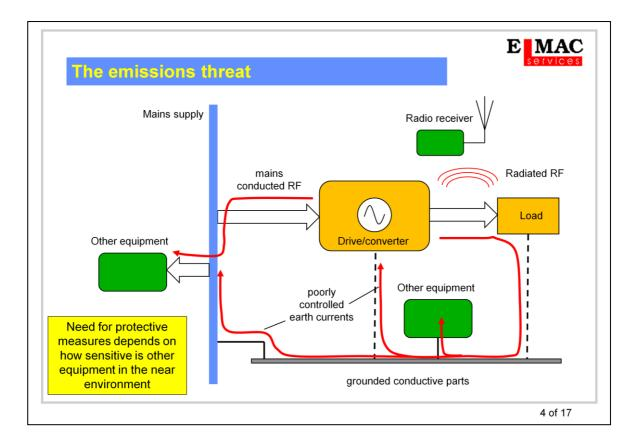
The drive or converter itself is not an important source of direct emission, because its dimensions are much less than a half wavelength over the relevant frequency range. There may be strong fields close to the unit's housing, which can be seen by near-field probing, but they diminish rapidly with increasing distance. On the other hand the power wiring can be extensive and may form an effective antenna for the generated frequencies.
