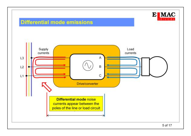
Before considering mitigation measures, it is necessary to be clear on the difference between differential and common mode emission paths. Mitigation for one mode will be ineffective for the other; sometimes both modes must be treated by separate methods.
