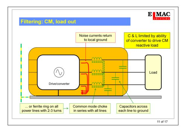
Common mode filtering can also be applied to the output. As with the differential mode filter it is necessary to be sure that the filter parameters are matched to the output of the drive or converter module. The principle is that common mode currents are returned to the module's local earth terminal before they pass out into the cable to the load, by the capacitors; and the choke offers a higher impedance to these currents before they pass to the cable, attenuating them further.
