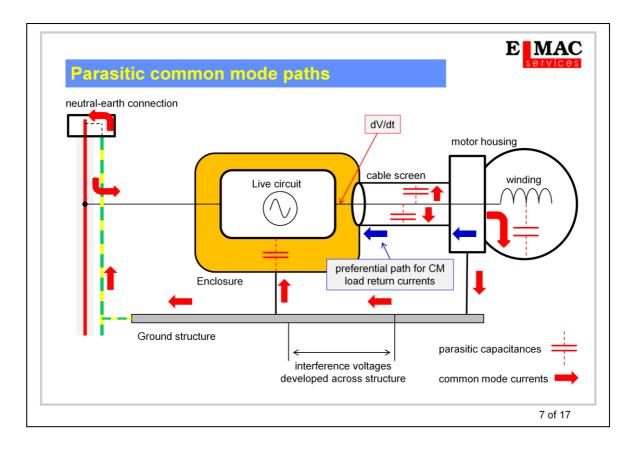
The main cause of high frequency common mode emissions is the current flowing from the output terminals to earth through the capacitance of the load cable and the load parasitics (in the case of a variable speed drive, the motor winding-to-case capacitance) to earth. In many converter and drive applications, the output is switched in PWM fashion with the full dV/dt being passed to the load.
