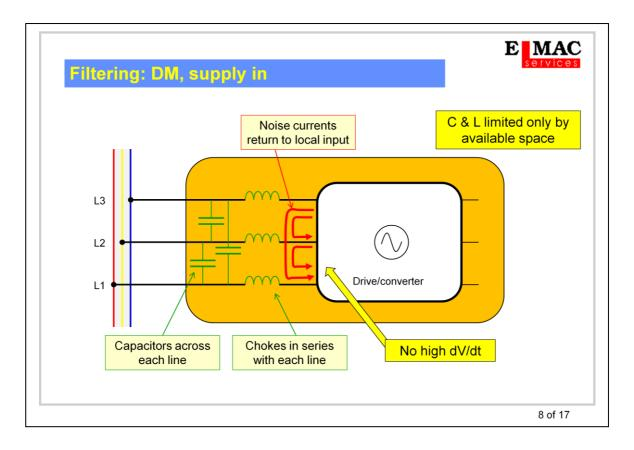
Differential mode filtering at the input of a switching converter is straightforward to implement, involving capacitors between each line and separate chokes in series with each line, without any connection to an earth point. Here, the filter capacitors are subject only to the input voltage waveform, which may be DC or 50/60Hz AC in most applications.
