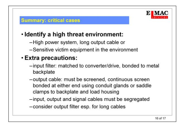
In a more complex environment or with high power systems then full precautions need to be taken. A complex victim environment includes AM broadcast and short wave radio receivers, analogue instrumentation using very low signal levels (thermocouples, resistance sensors, strain gauges), wideband/fast circuits such as audio or video systems, or unscreened digital data links. All such items are likely to be affected by the harmonic noise generated by the switching converter output.
