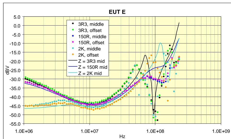
EUT A: 3 ohms resistive, EUT B: 2K ohms resistive, EUT C: 200pF capacitive, EUT E: 40 $\mu$ H inductive; ◆ or ▲ symbols show measurement, continuous line shows model
