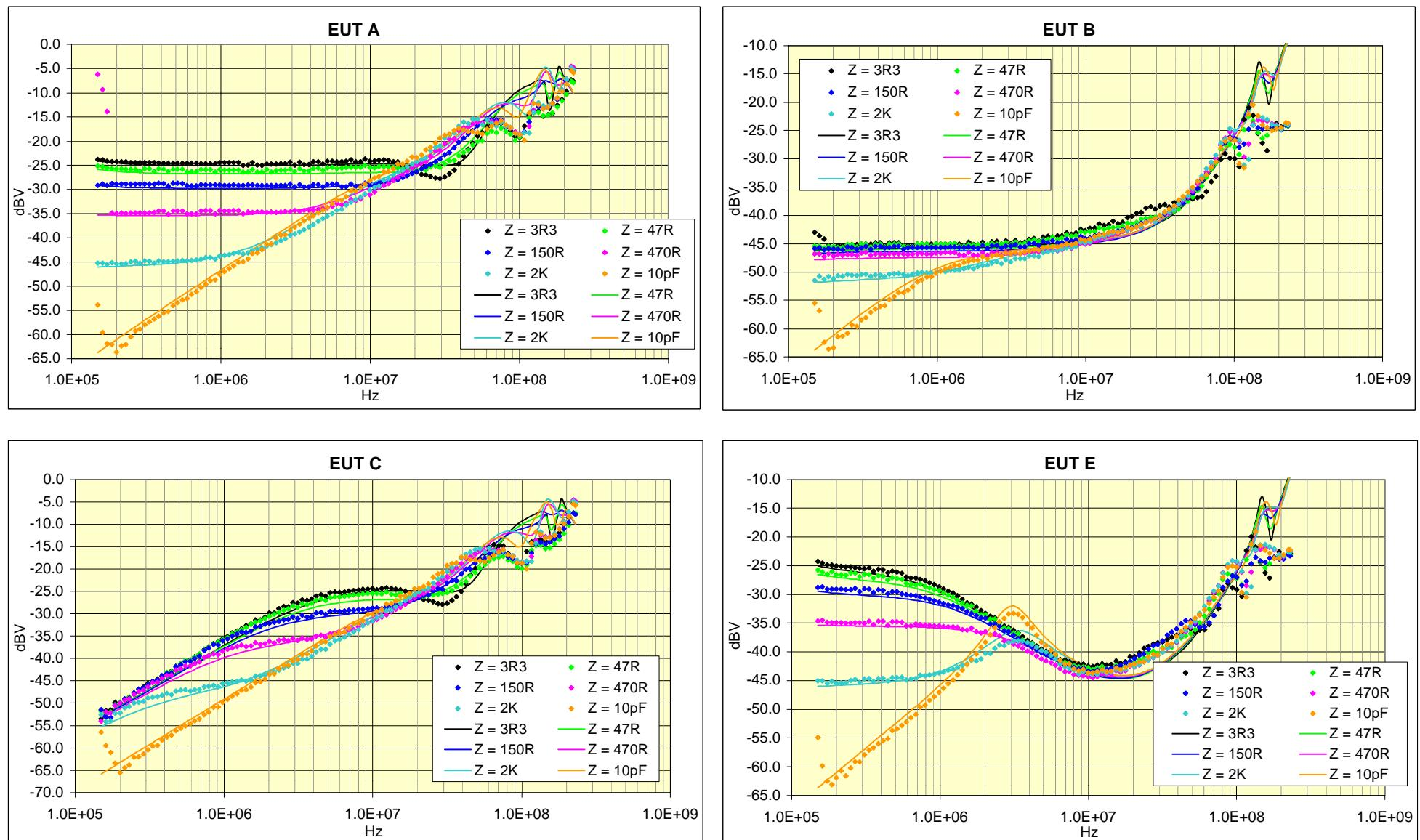
EUT A: 3 ohms resistive, EUT B: 2K ohms resistive, EUT C: 200pF capacitive, EUT E: 40μH inductive; ◆ or ▲ symbols show measurement, continuous line shows model
