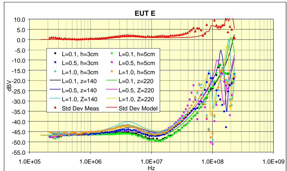
EUT A: 3 ohms resistive, EUT B: 2K ohms resistive, EUT C: 200pF capacitive, EUT E: 40 $\mu$ H inductive;  $\blacklozenge$  or  $\blacktriangle$  symbols show measurement, continuous line shows model
