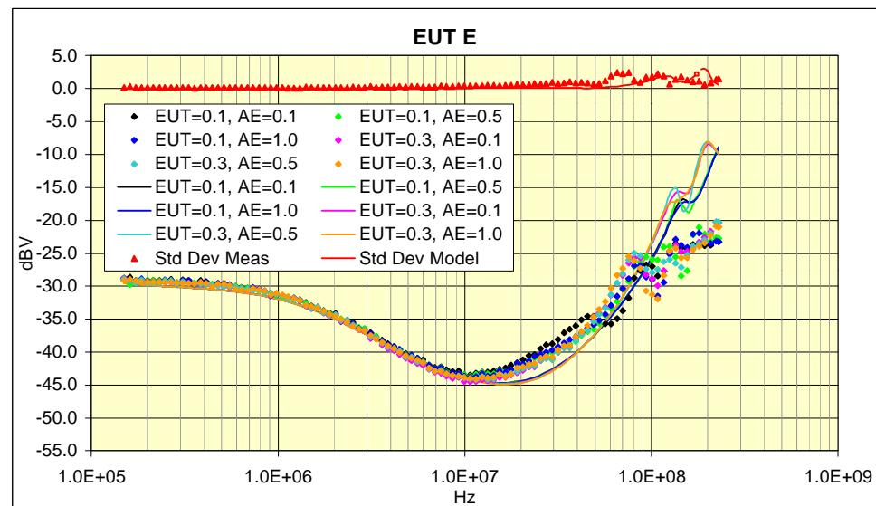
EUT A: 3 ohms resistive, EUT B: 2K ohms resistive, EUT C: 200pF capacitive, EUT E: 40 $\mu$ H inductive; ♦ or ▲ symbols show measurement, continuous line shows model
