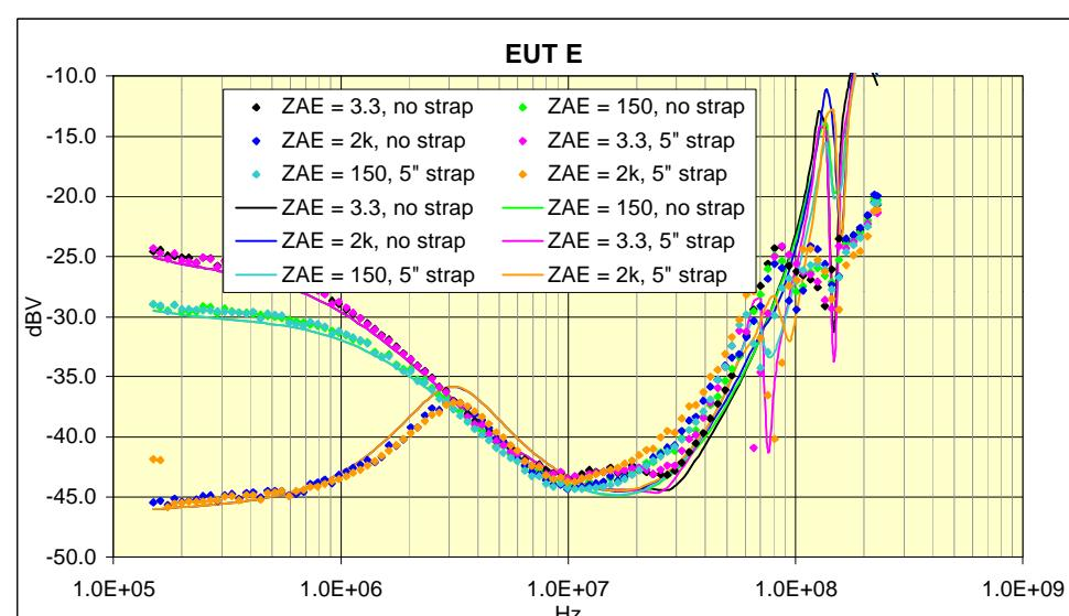
EUT A: 3 ohms resistive, EUT B: 2K ohms resistive, EUT C: 200pF capacitive, EUT E: 40μH inductive; ◆ or ▲ symbols show measurement, continuous line shows model
