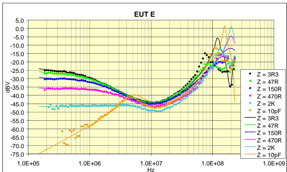
EUT A: 3 ohms resistive, EUT B: 2K ohms resistive, EUT C: 200pF capacitive, EUT E: 40uH inductive; ◆ or ▲ symbols show measurement, continuous line shows model
