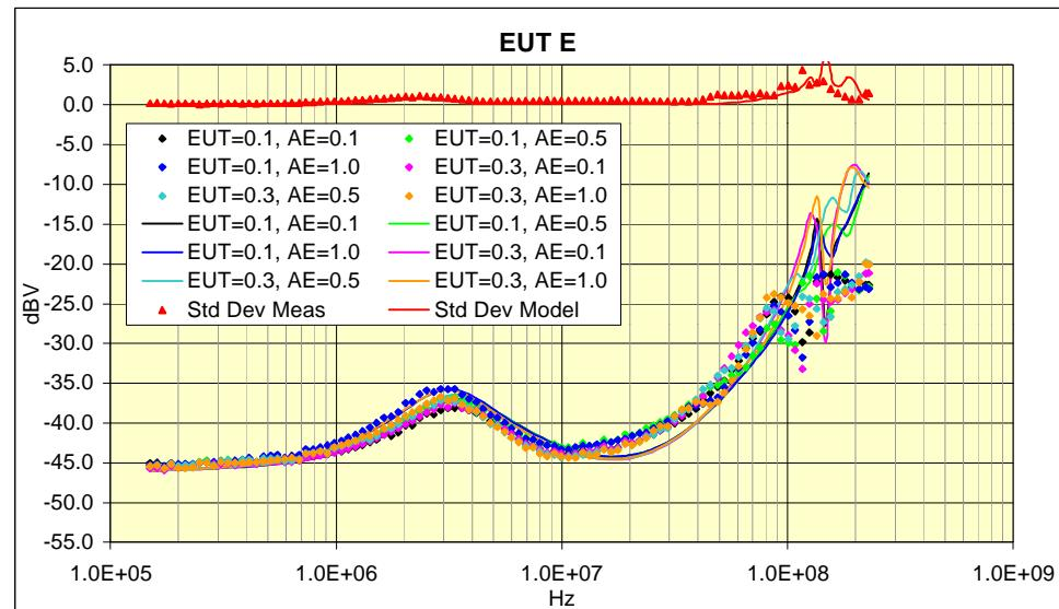
EUT A: 3 ohms resistive, EUT B: 2K ohms resistive, EUT C: 200pF capacitive, EUT E: 40 $\mu$ H inductive;  $\blacklozenge$  or  $\blacktriangle$  symbols show measurement, continuous line shows model
